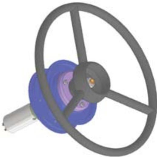
Figure 1: The electromechanical part of the farm tractor mechatronic steering module
