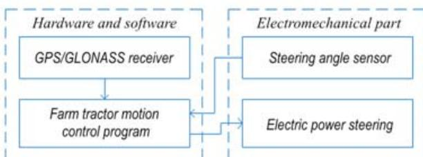
Figure 2: Mechatronic module functional diagram
