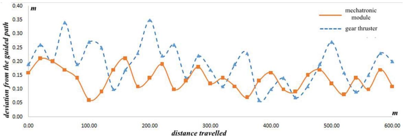
Figure 9: Deviation from the guided path of the farm tractor with the mechatronic module and the gear thruster
